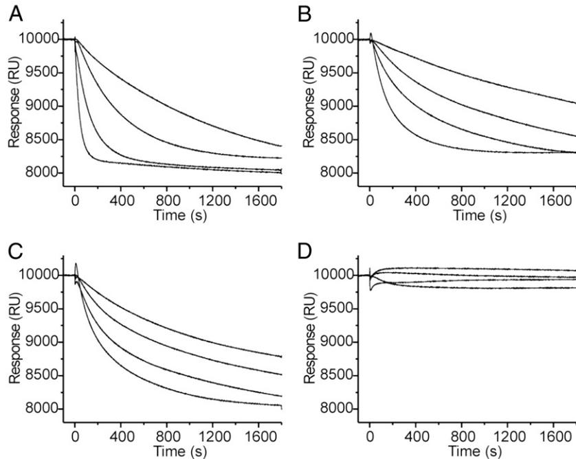
Fig. 5. Extraction of CHO from liposomes of various compositions. The liposome covered surface of L1 chip was prepared as described in the legend to Fig. 3. The cholesterol was extracted with 0.25, 0.5, 1 and 2 mM MBCD (curves from top to bottom) at  $2 \mu\text{l}/\text{min}$  for 30 min. (A) DOPC:SM:CHO 70:0:30; (B) DOPC:SM:CHO 53:17:30; (C) DOPC:SM:CHO 30:30:40; (D) DOPC:SM:CHO 40:40:20. The sensorgrams for DOPC:SM:CHO 17:53:30 looked similar to those presented in panel D.
